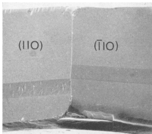
Figure 4 (110) and (\bar{1}\bar{1}0) cleavage faces of specimen A viewed along [0\bar{1}0] . Etched 12 min in AB etch. SEM micrograph, \times 130 .
